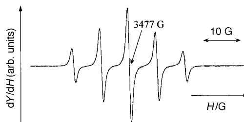
Fig. 7 EPR Spectrum recorded at room temperature for o -NITBAH into solution ( 5 \times 10^{-4} \text{ M} in \text{CH}_2\text{Cl}_2 ). The simulated spectrum ( g = 2.0065 , a_{\text{N}} = 7.59 \text{ G} , individual line width 0.8 lorentzian/gaussian shape: \Delta B = 1.18 \text{ G} ) is superimposed on the experimental spectrum.
